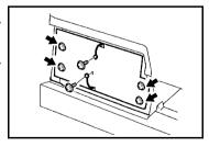
Remove the CCD Assy Lower Plate. (2 screws)
